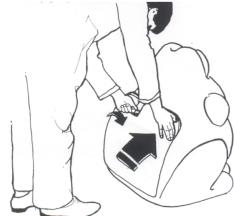
Simply push door panel back into its original position and lock with special key provided.
