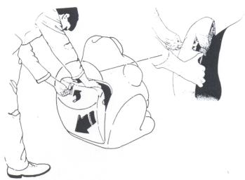
1 Using the key provided unlock and pull door away from main body. The door can then be lifted off using the hand holes provided.
